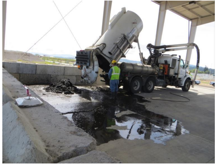
Dewatered materials drain into adjacent settling pool. Water from pool then passes through an oil/water separator, followed by a sand filter bed, and then to a bio-infiltration pond. Photo credit: City of Spokane Decant Facility
