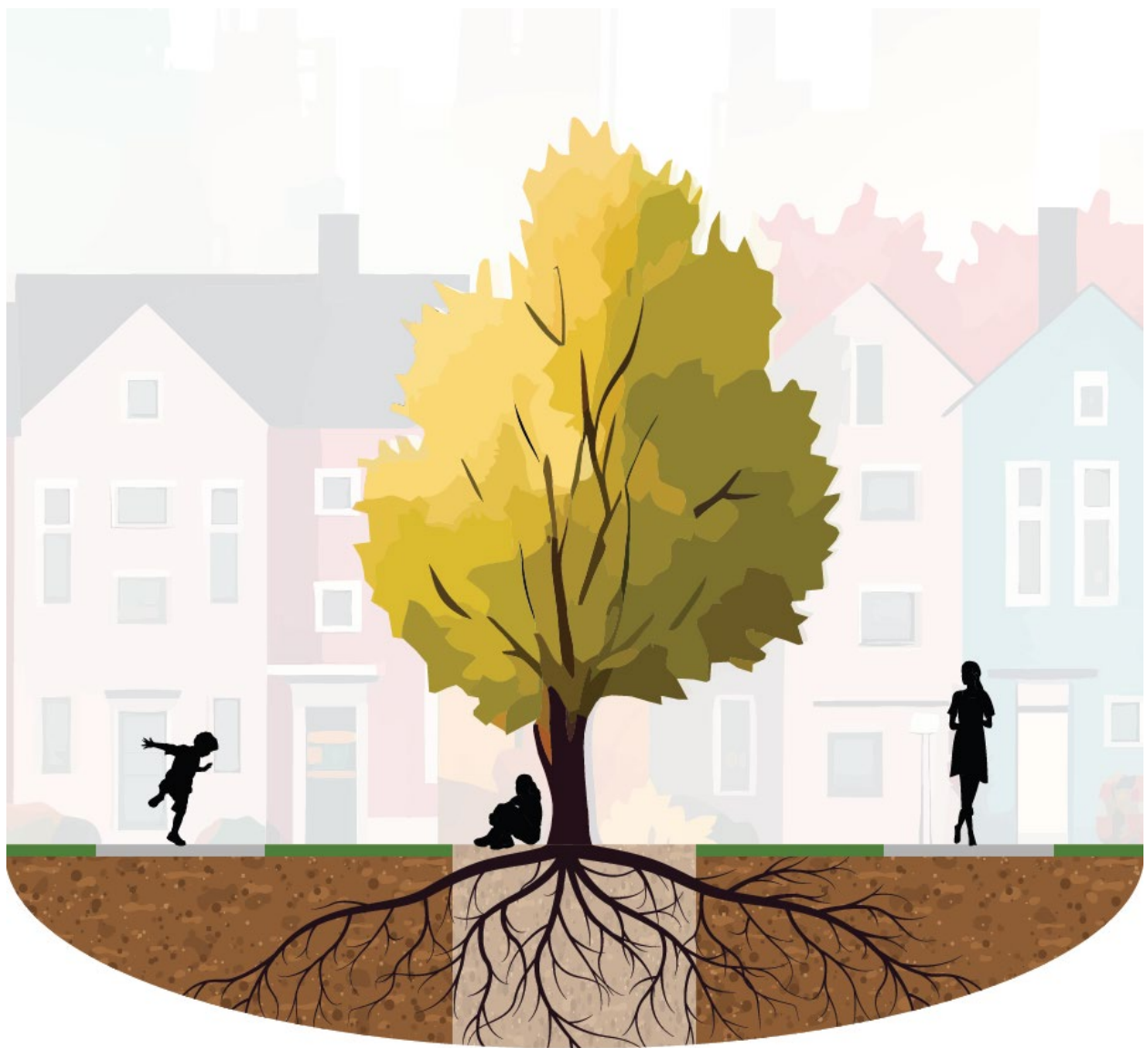
Figure 9: Uncovered planting pits are implemented in areas with adequate space to increase tree performance and decrease damage to neighboring infrastructure.
