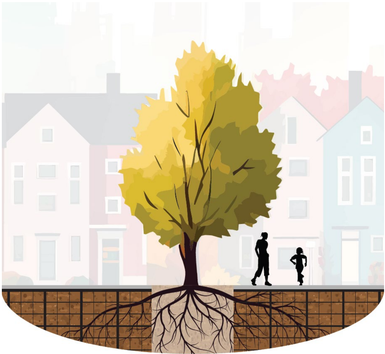
Figure 3: Suspended pavements utilize a network of pillars or cells to transfer weight from the load-bearing pavement above the tree's root system to a sub-base below it, keeping the soil in between uncompacted and available for the tree's use.
