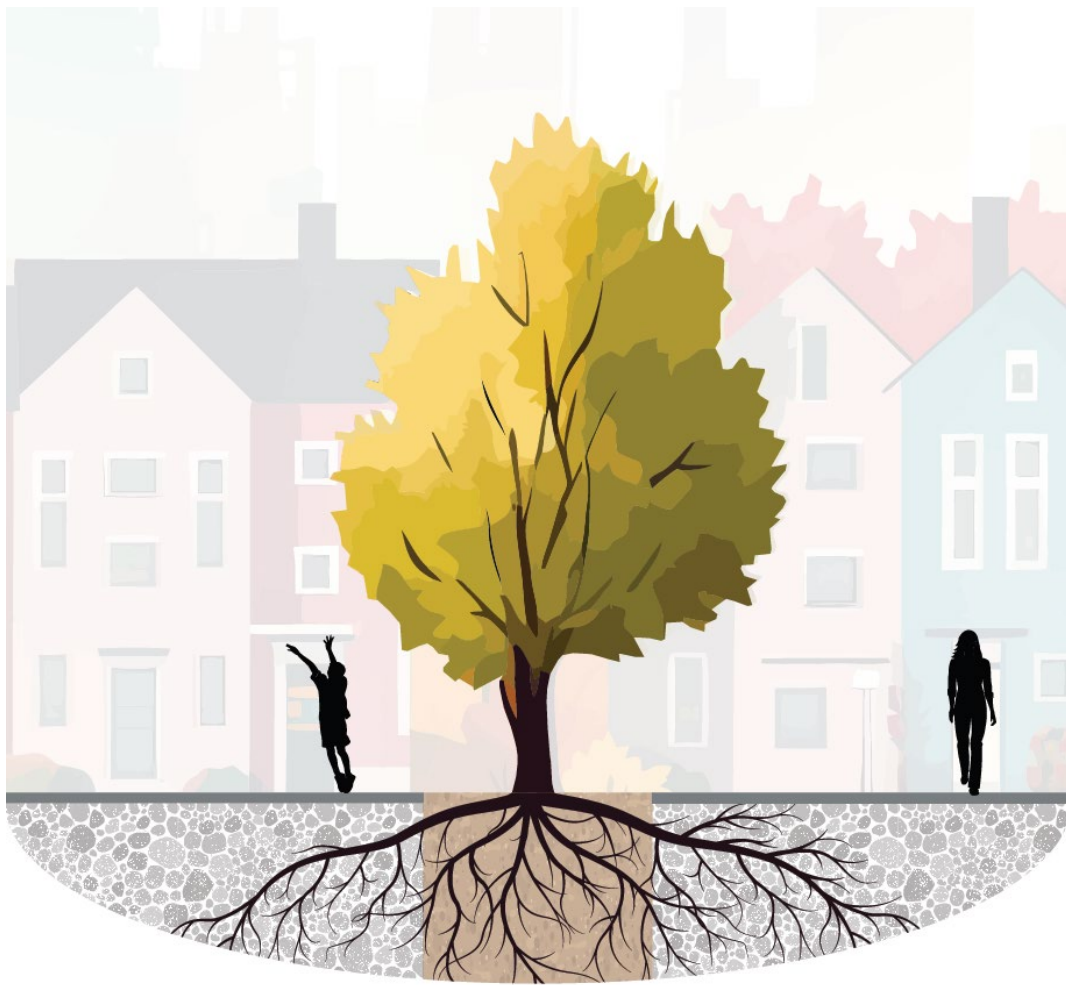
Figure 7: Structural soils allow trees to survive in paved urban areas by mixing load-bearing stone particles into the soil at a ratio of approximately 80% stone to 20% soil.
